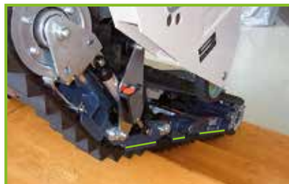
Easy and safe landing by flexible frame
