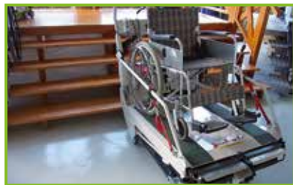
Easy and safe landing by flexible frame
